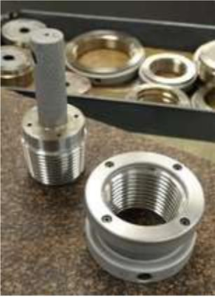
Hemco Gage manufactures precision gages for the petroleum industry, including this thread plug and ring.
